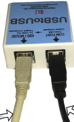
This port is also to be plugged into the computer running the USBtoUSB.exe configuration program.
